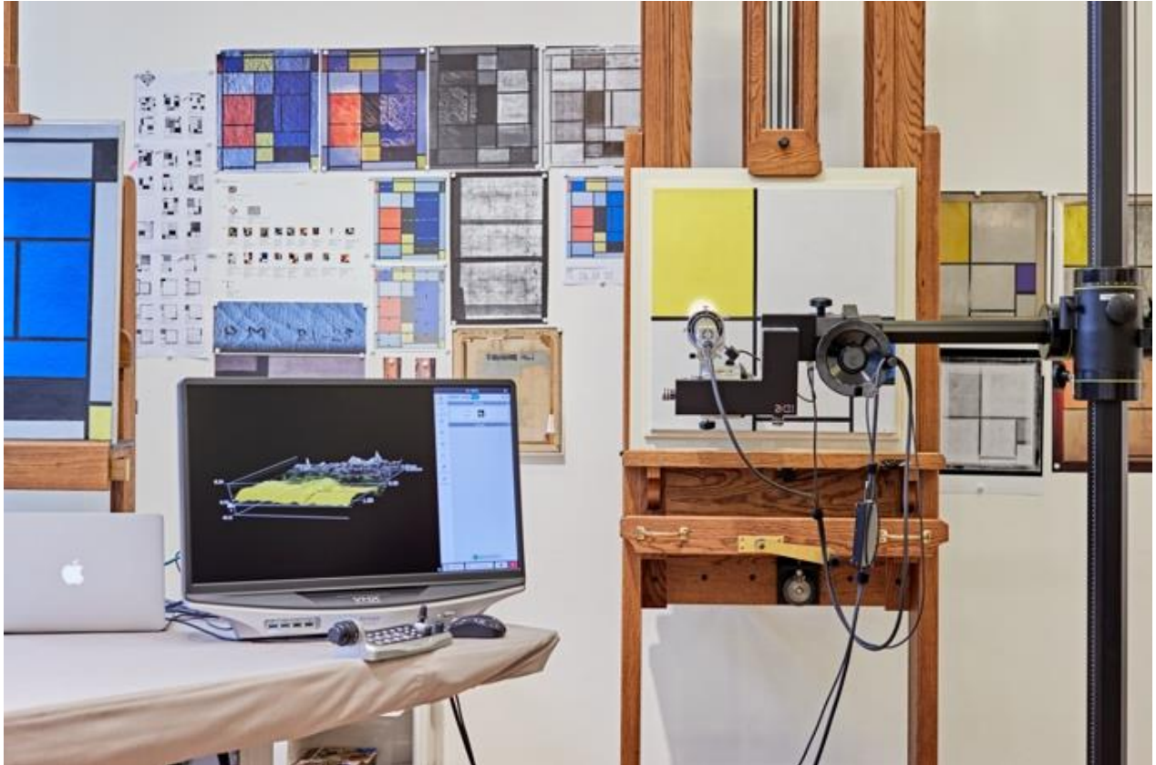
Abb. 3 Complete setup with Keyence VHX-7000, IDC multi-axes head und FOBA stand Piet Mondrian, Composition with yellow and blue , 1932, Fondation Beyeler, Riehen/Basel, Collection Beyeler
